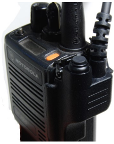
Attach accessory connector to portable radio
