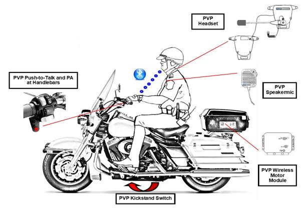
KICKSTAND UP = Mobile Radio Receive/Transmit
