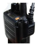
Attach accessory connector to portable radio.
