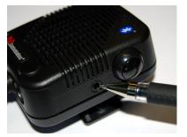
2) Use a pen (or similar item) to press the interior mounted pairing switch for 2-3 seconds until the shouldermic LED transitions to a solid color, then release. The wireless device will now power off.
