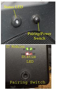
3) Verify motor kit still has power connected to it (ignition turned on or mobile radio turned on, etc.) Power off the motor kit by pressing the pairing switch — same procedure for power down as step 2.
